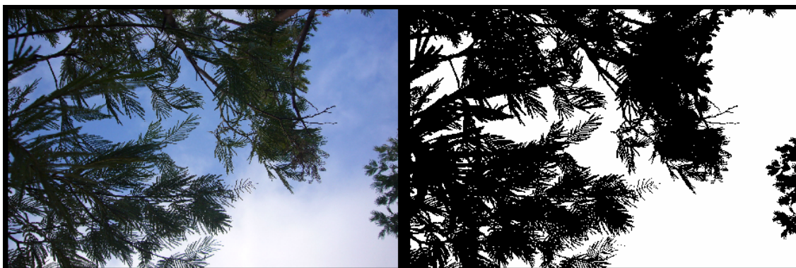
Figure 2: Example of the quantitative field measurements of PPC from upward looking photos. Photos (left) were classified (right) into canopy elements (black) and sky (white). PPC corresponds to the relative area of canopy elements in the classified photo (0.49 in this example)
