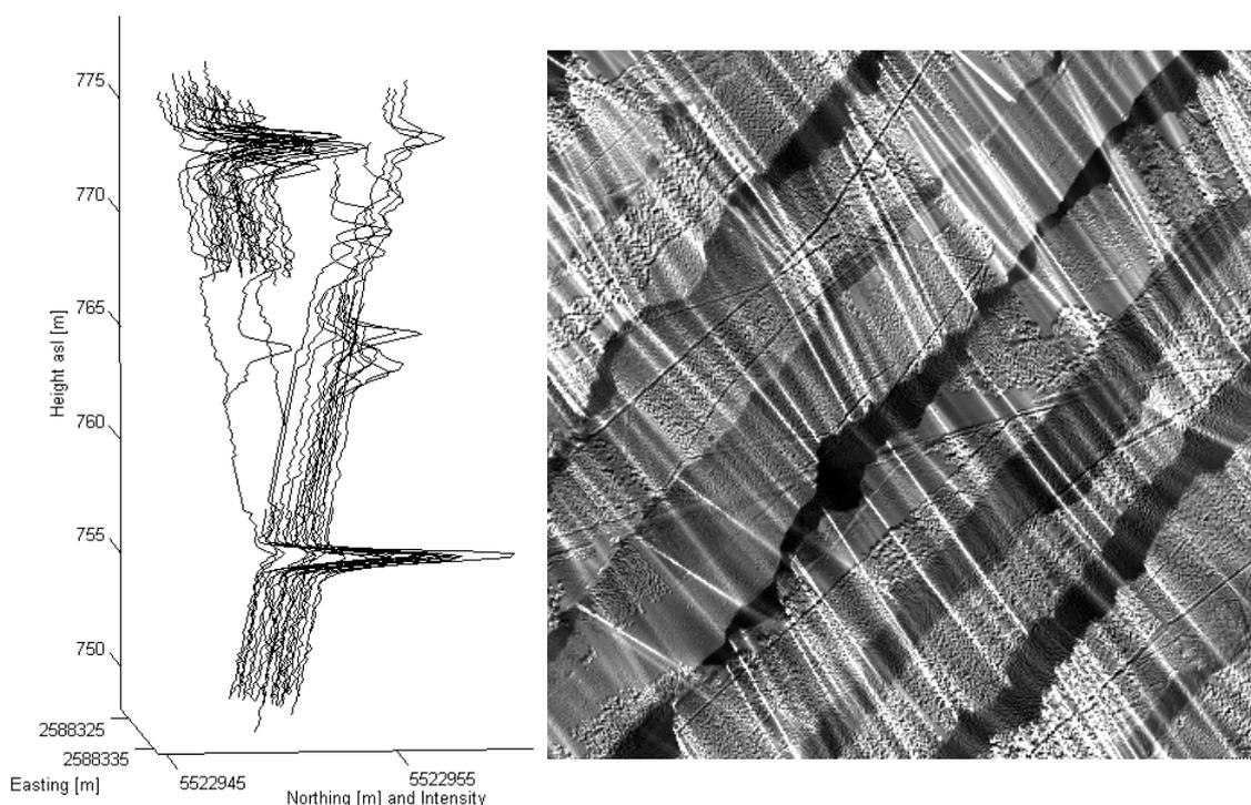
Figure 1: Left: Full waveforms from two flight lines converging on a small ground area. The ground level is at about 756 m asl where the lowest peaks occur. Right: Frequency of laser hits in an area of 400 x 400 Pixels; flight line overlapping and aircraft motions can be seen.
