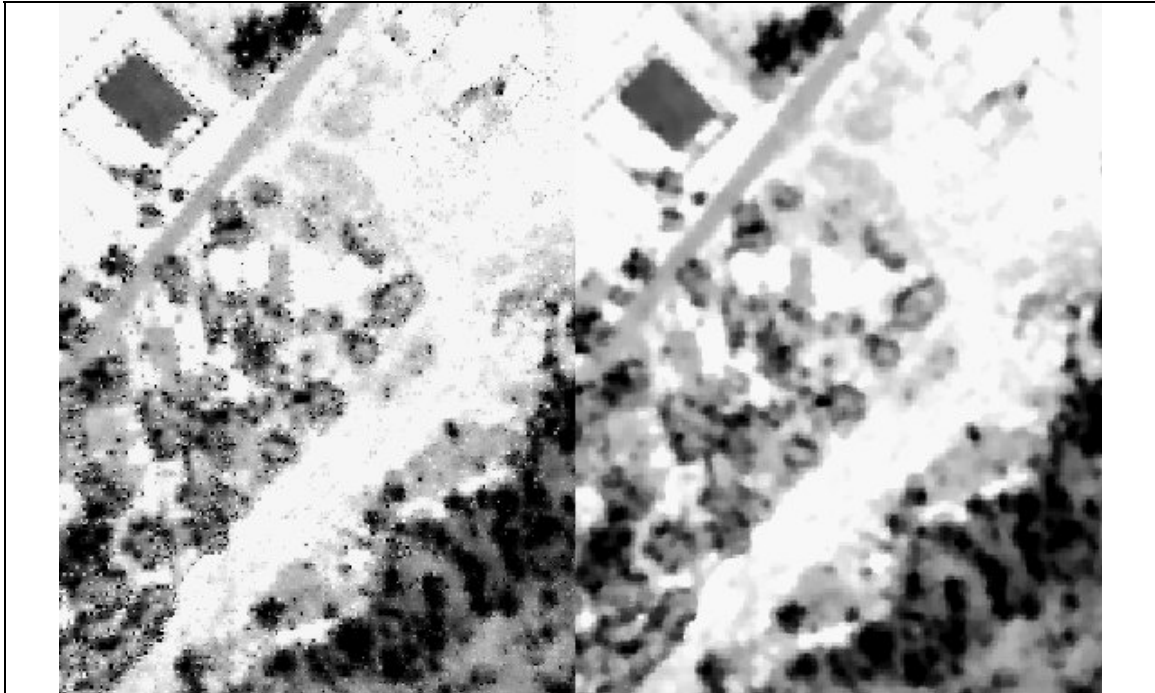
Figure 1: Intensity image generated using normal core interpolation (left) and intensity image filtered using a median filter (right)
