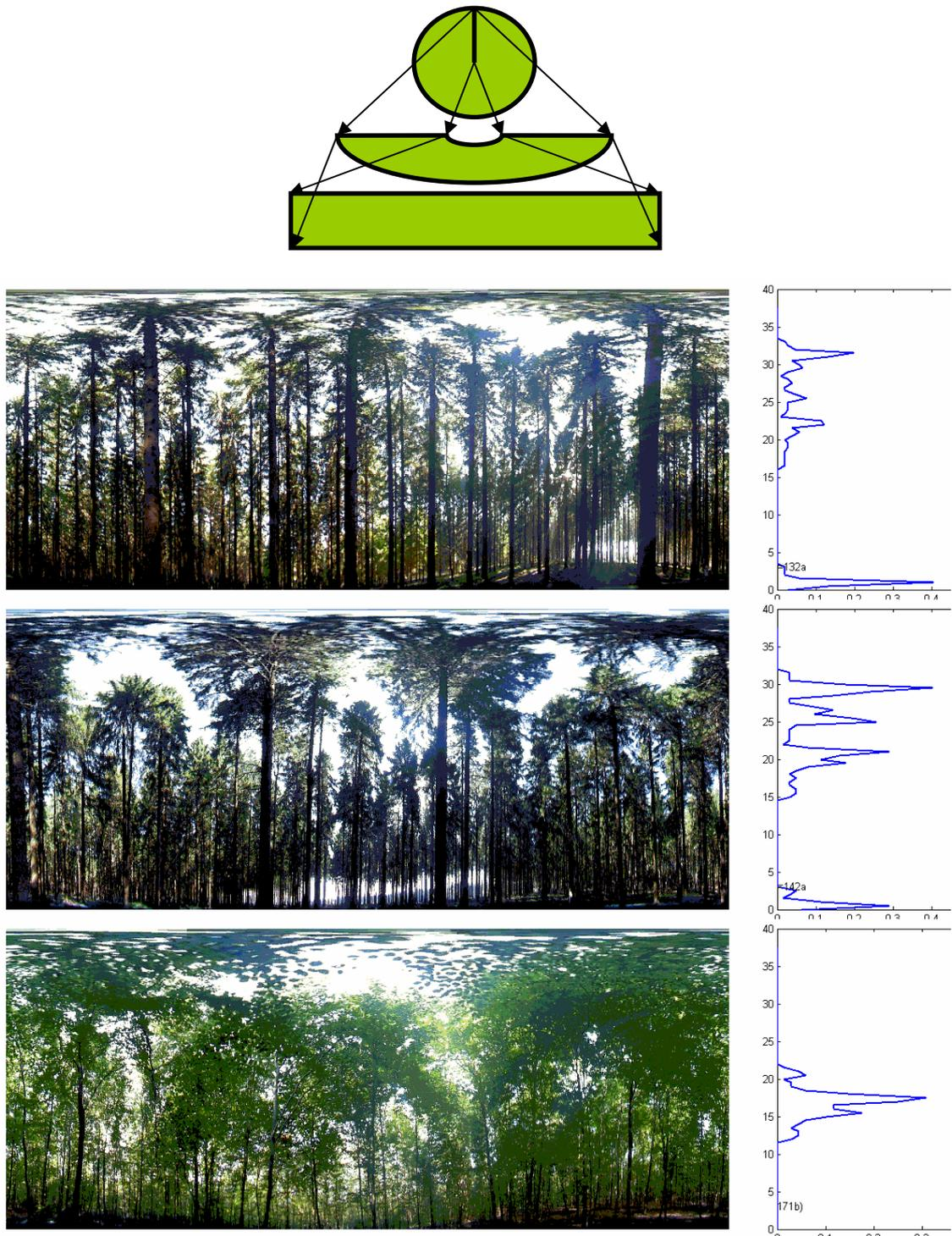
Figure 4: Unrolled hemispherical photos and corresponding ALS height profiles
